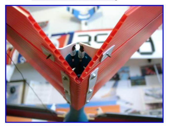
Fold the tail and mount at a 90 degree angle. Make sure hinge line clears the end of the fuselage. Position and location of the screws is not critical as long as the tail is square and secure. Notice how control horns are positioned for proper clearance. When making horns for the elevators and ailerons, make sure and make right and left ones. Take care that the elevator pushrods do not hit the self tapping screws inside the fuselage.
